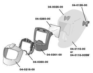
04-0016-(filter options) Complete Speedglas FlexView system 04-0016-00 Complete Speedglas FlexView system with no filter Add "SW" for SideWindows option.
